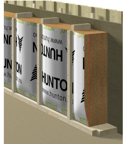
Illustration shows wall insulated with Nativo Wood Fibre Blown-In Insulation.
